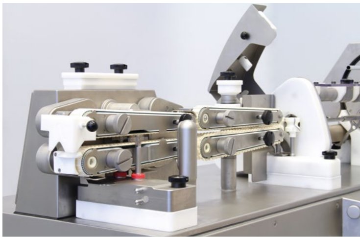
↑ Separating with 2-belt solution and sensor
